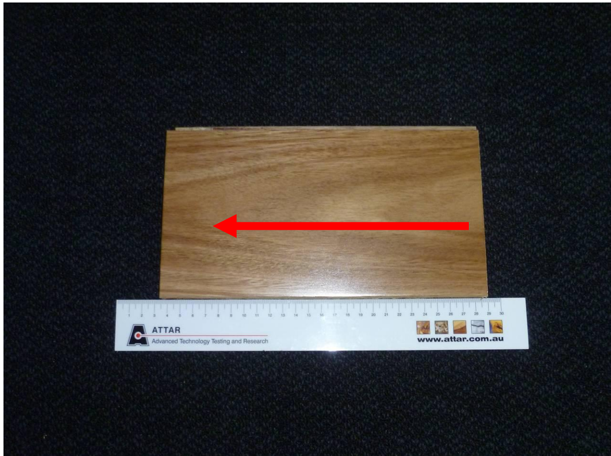
Figure 1: Big River Engineered Pre Finished Flooring. Arrow indicates direction of test.
